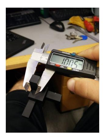
This year the 3D printing facility of SDU campus Sonderborg got a lot of request about precision of hobby machines we are using. In case to determine the precision the testing procedure was developed and testing was made. The steps of testing are following:
